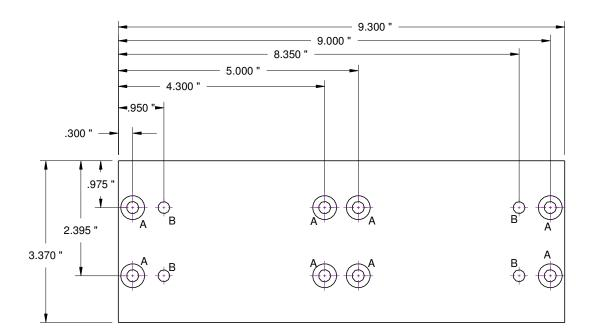
A Counter bore for 1/4-20 Button Head .257 " thru B Tap 1/4-20 Thru
